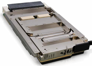
Figure 3: VPX3-1262 in Conduction-cooled with high-performance heat pipes
