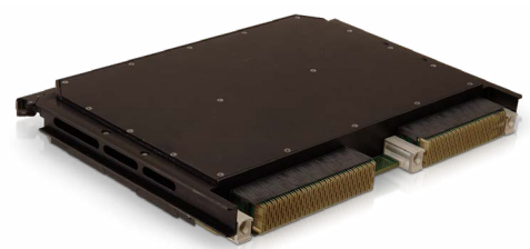
Figure 4: CHAMP-XD4 in VITA 48.8 Air Flow Through (AFT) Cooling
