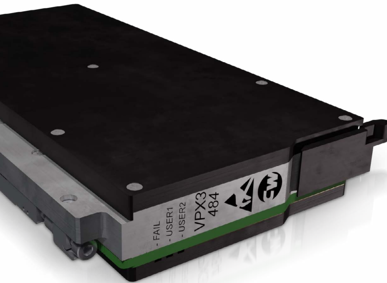
Figure 1: CHAMP-XD3 (VPX3-484) 3U VPX High Performance Processor Card with Enhanced TrustedCOTS
