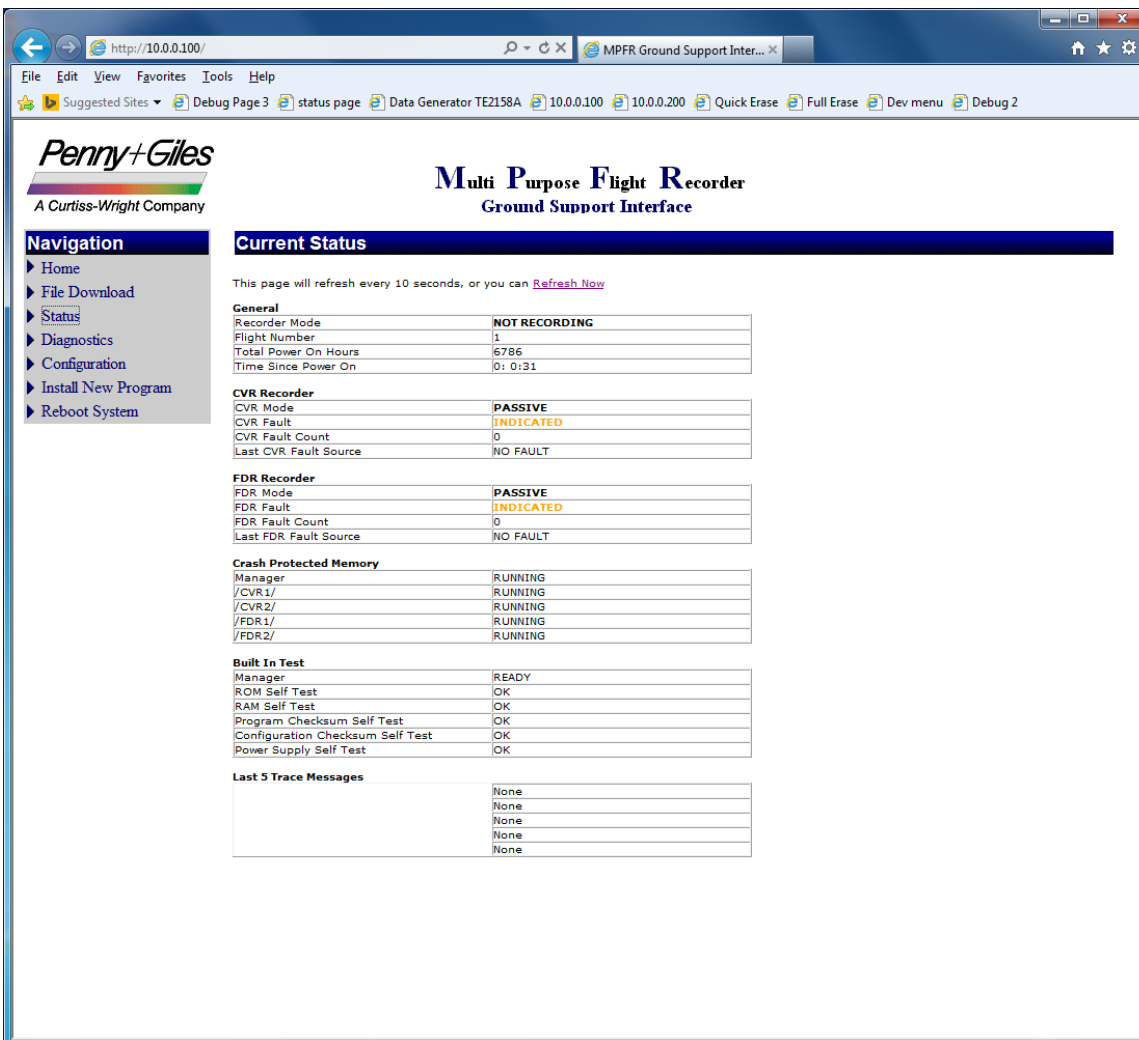
Figure 13 MPFR Ground Support Interface
